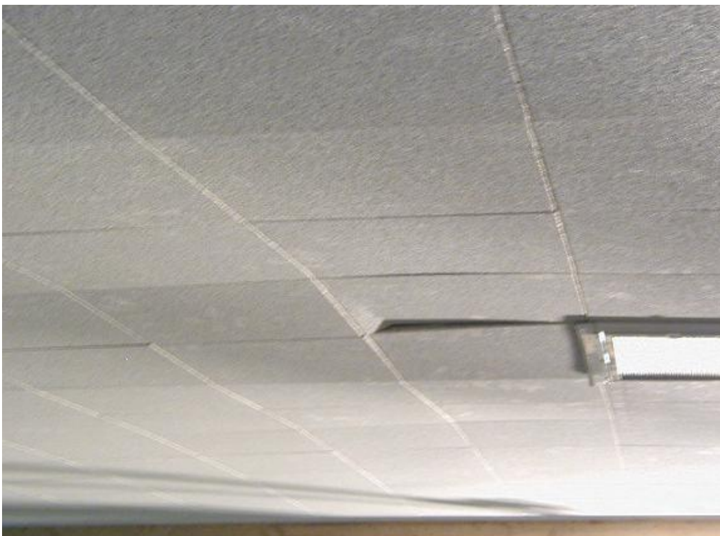
Figure 3-1. Displacement of perimeter tiles over perimeter spring clips following Test 20 for ceiling system CS1.
